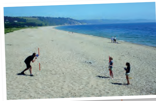
Using a clinometer and ranging poles to measure the angle of a beach profile.
