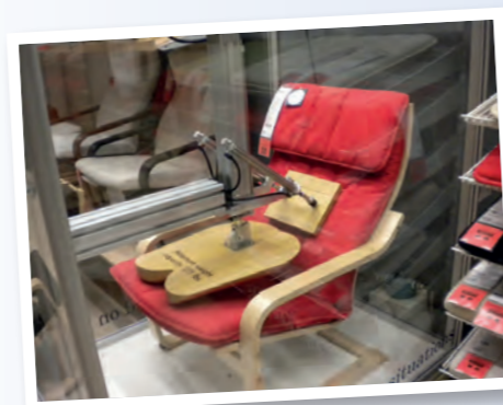
Testing a chair using high-pressure pneumatics to assess its strength under different weights
