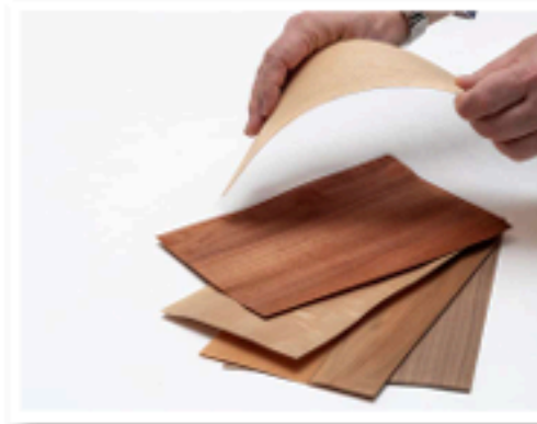
Thin sheets of wood veneer can be applied to most manufactured boards giving these materials the appearance of solid wood, achieved at a much lower cost.
